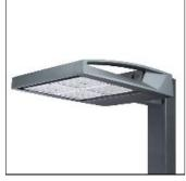
Choice of 16 high-efficiency, patented AccuLED Optics™, 3,400 - 61,800 lumens, up to 131 lp/W, Standard in 4000K CCT, 70 CRI, optional 2700K, 3000K, 5000K and 6000K, -40°C to 40°C operating range, 120-277V 50/60Hz, 347V 60Hz or 480V 60Hz operation, IP66 rated housing and LED Light Squares, Thermally conductive polymer heatsink for up to 22% weight reduction, Pole, mast-arm or wall-mounted configurations, 3G vibration rated, Five-year warranty
