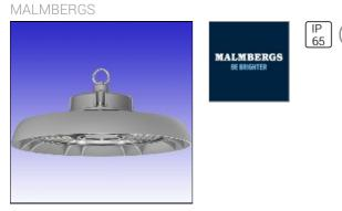
Industrial luminaire 4000K 100W D-marked, IP65, 230V Range of uses: Indoor areas. Mounting: Mounting bracket in robust steel, for surface mounting through holes or wire mounting. Connection: Cable inlet ready with 0,3m 3G1,0mm<sup>2</sup> H07RN-F through cable gland M16. Description: Grey body made of die cast aluminium. Weight: 1.5 kg Dims ØxH: 260X100 . Protection class: IP65.
