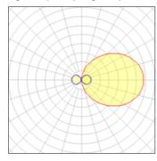
LED CCT 6000 K Lamp type Nominal lamp power 15 W CRI 70 Total flux 100% 589 lm LOR Luminous efficacy 39 lm/W ULOR 50% Total power 15 W
