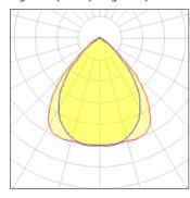
Lamp type LED CCT 4000 K Nominal lamp power 28 W CRI 80 Total flux LOR 100% 3500 lm Luminous efficacy 125 lm/W Total power 28 W
