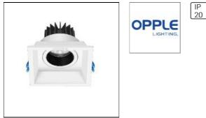
Housing:Aluminium; Mounting ring: white; Installation: recessed; Dimensions:105\*105\*75.5; Ceiling cutouts:Ф95\*95; Power:9W; Power factor:0.9; Efficacy : 65Lm/w Colour temperature:4000K; Colour rendering:RA90; Beam angle:15°; Total luminous flux of luminaire:585Lm; Service life:30,000h; Degree of protection:IP20;
