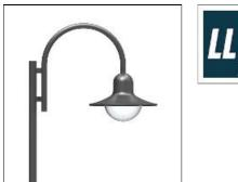
For medium light requirements, mounting height 3.50 - 4.00 m. - Impact-resistant clear or beaded polycarbonate attachment, UV-stabilized -Special reflector of premium highest-grade aluminium, burnished and anodized, for excellent illumination and glare protection - Aluminium
