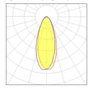
Lamp type LED CCT 2700 K Nominal lamp power 10 W CRI 80 Total flux LOR 100% 560 lm Luminous efficacy 56 lm/W Total power 10 W
