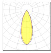
Lamp type LED CCT 3000 K Nominal lamp power 15 W CRI 90 Total flux LOR 100% 1157 lm Luminous efficacy 77 lm/W Total power 15 W
