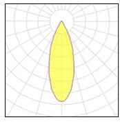
Lamp type Nominal lamp power Total flux Luminous efficacy LED 33 W 2850 lm 86 lm/W
