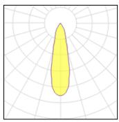
Lamp type LED CCT 4000 K CRI Nominal lamp power 45.8 W 90 Total flux 5410 lm LOR 100% Total power Luminous efficacy 118 lm/W 45.8 W
