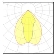
1 x LED Nominal lamp power 55 W LOR 83% Lamp flux 6950 lm Total flux 5785 lm Luminous efficacy 126 lm/W Total power 60 W CCT 4000 K CRI 80
