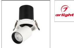
Recessed rotating retractable ceiling light. Power 10 W, luminous flux 900 lm, 90 lm/W, warm 3000 K, CRI>90, angle 24°, supply voltage 230 V. White round aluminum housing, PC screen, protection degree IP20. Size (ØL×H) 105×127 mm. Recessed installation, installation hole Ø 95 mm. Driver 30-48 V, 250 mA, ripple <1%.
