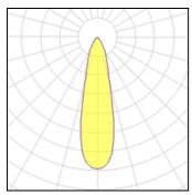
Lamp type LED CCT 3000 K Nominal lamp power 45.8 W CRI 90 Total flux 5130 lm LOR 100% Luminous efficacy 112 lm/W Total power 45.8 W
