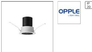
Housing:Corrosionresistant Cast Aluminium; Installation: Recessed; Dimensions:D68\*H68mm; Ceiling cououts:Ф55mm; Power:5W; Power factor:0.5; Efficacy:70Lm/W; Colour temperature:3500K; Colour rendering:Ra>90; Beam angle:50°; Total luminous flux of luminaire:350Lm; Service life:30000h; Degree of protection:IP20;
