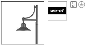
IP66, Class I. IK10. Marine-grade die-cast aluminium alloy. 5CE superior corrosion protection including PCS hardware. Silicone rubber gaskets. Polycarbonate main lens. LED modules can be easily removed for updating. CAD-optimised optics for superior illumination and glare control. OLC® One LED Concept. Recommended mounting height 3,0-4,5 m, depending on lamp type selected. Brackets to be ordered separately.
