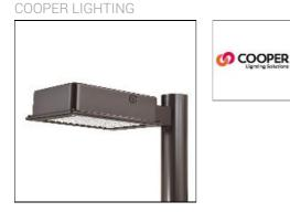
One-piece, die-cast aluminum housing can be pole or wall-mounted, Optical design creates consistent distribution and scalability, Choice of 12 high-efficiency, patented AccuLED Optics™, Standard in 4000K (+/- 275K) CCT and nominal 70 CRI, Suitable for operation in -40°C to 40°C ambient environments, 120-277V 50/60Hz, 347V 60Hz or 480V 60Hz operation, Proprietary circuit module withstands 10kV of transient line surge, Optional battery pack and bi-level switching, Five-year warranty
