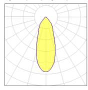
Lamp type LED CCT 3000 K Nominal lamp power 7.5 W CRI 80 Total flux LOR 100% 430 lm Luminous efficacy 57 lm/W Total power 7.5 W
