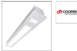
Recessed grid 8" on center. Use the DFCL for hard ceilings, 7.5W maximum LED MR16 reading light, with full rotation and swivel, Choose from 3 illumination levels for the ambient exam function, IP65 optional for dusts and water ingress protection, NSF listing and anti-microbial finish for sterile environments, Amber night light and several white color temperatures available, Low voltage relay available for pillow switch control, Emergency battery also available
