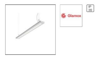
Light source: LED Lumen out: 3997 CRI: 80 Colour temperature: 3000 Total effect: 33 Lumen per watt: 120 Optic: WM Driver: DALI/HF Main body material: Steel IP class: 20 IK class: 3
