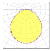
Lamp type LED CCT 4000 K Nominal lamp power 34.78 W CRI 80 Total flux 4666 lm LOR 100% Luminous efficacy 134 lm/W ULOR 3% Total power 34.78 W
