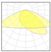
Lamp type Nominal lamp power Total flux Luminous efficacy LED 200 W 26200 lm 131 lm/W CCT CRI LOR Total power
