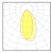
Lamp type LED CCT 3500 K Nominal lamp power 10.5 W CRI 83 Total flux 617 lm LOR 100% Luminous efficacy 59 lm/W Total power 10.5 W
