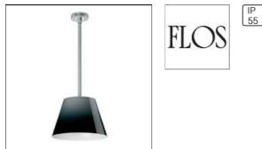
Ceiling luminaires for outdoor use providing direct and diffused light. Die-cast aluminum alloy wall or ceiling fitting with brillant finish. Injectionmolded polycarbonate (PC) cover rose. 316L stainless steel stem-polished. Opal-colored, vacuum-formed internal polycarbonate diffuser. Diffuser support in injection-molded opal colored polycarbonate. Crown support in injection-molded opal-colored polycarbonate. Two-color vacuum-formed engineering plastic outer crowns
