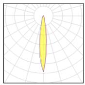
1 x LED Nominal lamp power 12 W LOR 69% Lamp flux 1620 lm Total flux 1124 lm Luminous efficacy 135 lm/W Total power 15 W CCT 3000 K CRI 80
