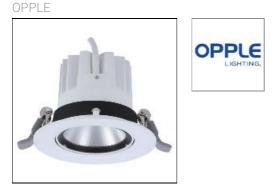
Housing: Aluminum+PC; Mounting ring: white; Installation: recessed; Dimensions: Φ85×57mm; Ceiling cutouts: Φ75mm; Beam angle: 36°; Lamp(s): LED; Power: 10W; Efficacy : 95Lm/w; Total luminous flux of luminaire: 950lm; Power Factor: 0.9; Mains voltage: 220-240V/50-60Hz; Colour temperature: 3000K; Colour rendering: Ra80; UGR: 22; IP/IK Grade: IP20; Class of protection II; Control System: on/off, DALI, 1-10V, BLE; Service life: 30,000h at 70% luminous flux;
