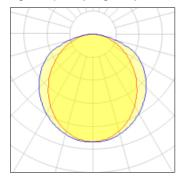
LED CCT 3000 K Lamp type Nominal lamp power 22.8 W CRI 85 Total flux 2051 lm LOR 100% Total power Luminous efficacy 90 lm/W 22.8 W
