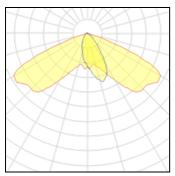
Lamp type LED CCT 3000 K Nominal lamp power 47 W CRI 80 Total flux 4650 lm LOR 100% Luminous efficacy 99 lm/W Total power 47 W
