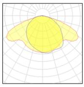
1 x Metal halide lampNominal lamp power15Lamp flux1500Luminous efficacy81 lrCCT290CRI1000
