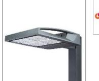
Choice of 16 high-efficiency, patented AccuLED Optics™, 3,400 - 61,800 lumens, up to 131 lp/W, Standard in 4000K CCT, 70 CRI, optional 2700K, 3000K, 5000K and 6000K, -40°C to 40°C operating range, 120-277V 50/60Hz, 347V 60Hz or 480V 60Hz operation, IP66 rated housing and LED Light Squares, Thermally conductive polymer heatsink for up to 22% weight reduction, Pole, mast-arm or wall-mounted configurations, 3G vibration rated, Five-year warranty
