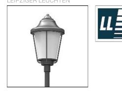
For medium light requirements, mounting heights from 3.00 - 4.00 m. - Excellent uniform illumination, optimal glare protection - Luminaire body made of aluminium/galvanized steel sheet - Impact-resistant opal polyethylene attachment, UV-stabilized - Steel tubing galvanized and painted - Adapter jack connection - Available in any RAL or DB colour without surcharge Voltage: 230V 50Hz Protected to: IP 55 Protection class: I/II Made to DIN VDE 0711 Luminaires generally compensated
