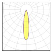
2700 K Lamp type LED CCT Nominal lamp power 2.75 W CRI 90 Total flux 186 lm LOR 100% Luminous efficacy 68 lm/W Total power 2.75 W
