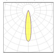
LED CCT 2700 K Lamp type Nominal lamp power 2.75 W CRI 90 Total flux 186 lm LOR 100% 68 lm/W 2.75 W Luminous efficacy Total power
