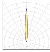
LED CCT 3000 K Lamp type Nominal lamp power 1 W CRI Total flux 76 lm LOR 100% Luminous efficacy 76 lm/W 100% ULOR Total power 1 W
