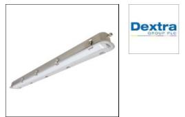
Splash LED - 1500mm, IP65 Corrosive resistant luminaire, with pressed stainless steel body and toughened polycarbonate diffuser. Options: E3 - Emergency control gear (480 lumens output) ST3 - Emergency Selftest AT3 - Emergency Autotest S - Switch Dimming D - Digital Dimming (DSI) A - Digital Addressable Lighting Interface (DALI) C - Bi-Level Dimming (Corridor Function) H - High Frequency Dimming (Analogue 1-10v) Available with glass cover on request
