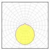
Lamp type LED CCT 3000 K Nominal lamp power 21 W CRI 80 Total flux 2640 lm LOR 100% Luminous efficacy 126 lm/W ULOR 15% Total power 21 W
