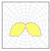
1 x Metal halide lamp Nominal lamp power 100 W LOR 55% ULOR Lamp flux 10000 lm 15% Luminous efficacy 47 lm/W Total flux 5462 lm CCT 3000 K Total power 115 W CRI 90
