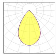
Lamp type LED CCT 3000 K Nominal lamp power 11.5 W CRI 80 Total flux LOR 100% 1150 lm Luminous efficacy 100 lm/W Total power 11.5 W
