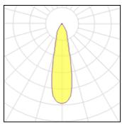
Lamp type LED CCT 3000 K Nominal lamp power 37.5 W CRI 90 Total flux 4320 lm LOR 100% Luminous efficacy 115 lm/W Total power 37.5 W
