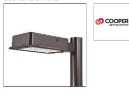
One-piece, die-cast aluminum housing can be pole or wall-mounted, Optical design creates consistent distribution and scalability, Choice of 12 high-efficiency, patented AccuLED Optics<sup>™</sup>, Standard in 4000K (+/- 275K) CCT and nominal 70 CRI, Suitable for operation in -40°C to 40°C ambient environments, 120-277V 50/60Hz, 347V 60Hz or 480V 60Hz operation, Proprietary circuit module withstands 10kV of transient line surge, Optional battery pack and bi-level switching, Five-year warranty
