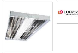
Durable CRS and alluminum housing with white enamel finish, High-Performance efficacy up to 170 LPW, LEDs available in 3500K, 4000K and 5000K at typical 85 CRI, Rated for -40°C to 55°C ambient, Lumen Maintenance – L84 @ 60,000 hours, Precision optics in narrow and wide distribution, Multiple lens options, Occupancy and daylight sensor for added savings, Up to 70% energy savings
