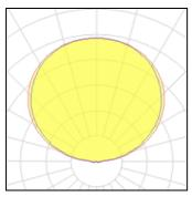
Lamp type I FD CCT 6500 K Nominal lamp power 0.6 W CRI 91 Total flux 4 lm LOR 100% Luminous efficacy 7 lm/W ULOR 97% Total power 0.6 W
