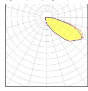
LED CCT 5700 K Lamp type Nominal lamp power 171 W CRI 70 Total flux 16644 lm LOR 100% Luminous efficacy 97 lm/W Total power 171 W
