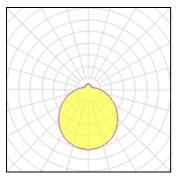
Lamp typeLEDCNominal lamp power32 WClTotal flux4060 lmLCLuminous efficacy127 lm/WUl
