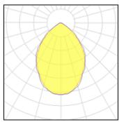
Lamp type Nominal lamp power Total flux Luminous efficacy LED 195 W 31320 lm 161 lm/W CCT CRI LOR Total power
