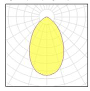
LED CCT 2665 K Lamp type Nominal lamp power 4 W CRI 85 Total flux LOR 100% 199 lm Luminous efficacy 50 lm/W Total power 4 W
