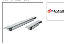
Cove lighting fixture with integral driver, Up to 1500 lm/ft (3 light level options at 500, 1000 and 1500 lm/ft), IP66 rated for continuity of lighting from interior to exterior spaces, 1% dimming, 0-10V (1% - 100%), 90 CRI standard, Up to 130 lm/W, Up to 300 ft run from a single power drop, Self-closing end cap + quick connects for easy error-free installation, Self-aligning brackets with 15 and 30 degree mounting angle options
