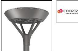
Die-cast aluminum housing and door, Lumens packages ranging from 3,000 - 29,000 lumens, Choice of 13 high-efficiency, patented AccuLED Optics™, Base casting slip fits over a standard 3" O.D. tenon, Wall, single and dual-mount configurations available, 10kV/10vkA surge
