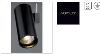
Shooter 1, Cylindrical Track Spotlight with 3-circuit Euro adapter, its simple and compact design is ideal for accent lighting; made of highquality, die-cast aluminum; chrome plated surface; lamp replace without tools by "Slide Change"; 3-phase adapter black; 1x max.50W QPAR16 GU10, 230V; 340 ° rotation and 90 ° tilt, IP 20;
