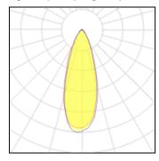
LED CCT 3000 K Lamp type Nominal lamp power 25.5 W CRI 92 Total flux 1821 lm LOR 100% Luminous efficacy 71 lm/W Total power 25.5 W
