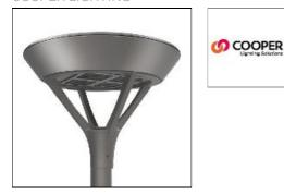
Die-cast aluminum housing and door, Lumens packages ranging from 3,000 - 29,000 lumens, Choice of 13 high-efficiency, patented AccuLED Optics<sup>™</sup>, Base casting slip fits over a standard 3" O.D. tenon, Wall, single and dual-mount configurations available, 10kV/10vkA surge protection standard, LED fixture features a five-year warranty
