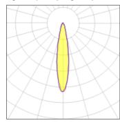
LED CCT 3000 K Lamp type Nominal lamp power 10 W CRI 80 Total flux LOR 100% 800 lm Luminous efficacy 80 lm/W Total power 10 W
